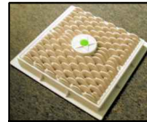
AquaStar WAV9, 9" X 9" Frame, Approved Max Flow Rate: Floor = 207 GPM @ 1.5 fps Wall = TBD 44.2 Sq In - Open Area V.G.B Approved Safety Drain
