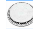
AquaStar 8AV, 8" Dia Frame, Approved Max Flow Rate: Floor = 88 GPM @ 3.2 fps Wall = 70 GPM @ 2.6 fps 8.8 Sq In - Open Area V.G.B Approved Safety Drain
