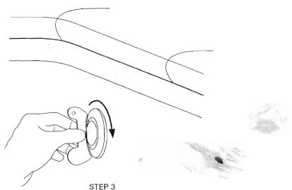
Using the lens wrench (part # 13.6151), thread the fixture into the wall fitting until it is snug.
